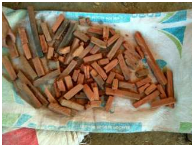
Figure 8 Damaging bricks for measuring the tensile strength
